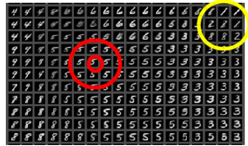
Figure 46: Illustration of how incremental learning is made possible through a topologically ordered prototype representation. Due to topological ordering, neighbouring prototypes are almost always situated in nearby regions of input space. Therefore, local updates of prototypes will almost always be local in input space as well, thus effectively enabling efficient incremental learning. This is shown here for a subset of prototypes trained on the MNIST database, the best-matching unit (BMU) for a "5" input being indicated by a small red circle. It is obvious that the local 2D update region, indicated by a larger red circle, is indeed local in the input space. The yellow circle indicates a region where this property does not hold (structural defect) but the reader can convince himself that this occurs but rarely.
