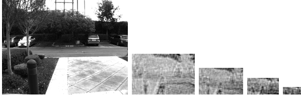
Figure 30: Topologically arranged pedestrian confidence maps as computed by the HOG+SVM method from the camera image (left). Confidence maps are computed on increasingly coarse spatial scales (from left to right), which allows to detect pedestrians of different sizes.
