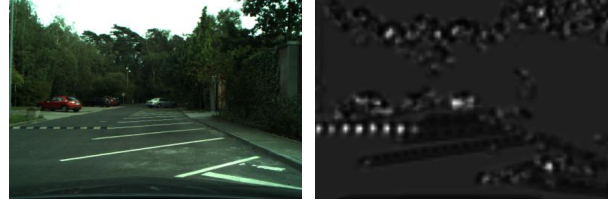
Figure 24: Example of how the appearance-based classifier works in the context-based object detection architecture: for each input image (a) , it produces a retinotopic, dense map of vehicle confidences (b) . This means that each pixel in this map represents the presence or absence of a vehicle, at a specific scale, centered on that pixel.
